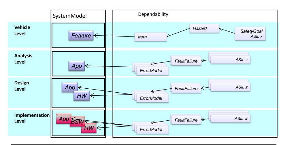
ErrorModel capture Failure propagation logic – can be identified using fault injection
