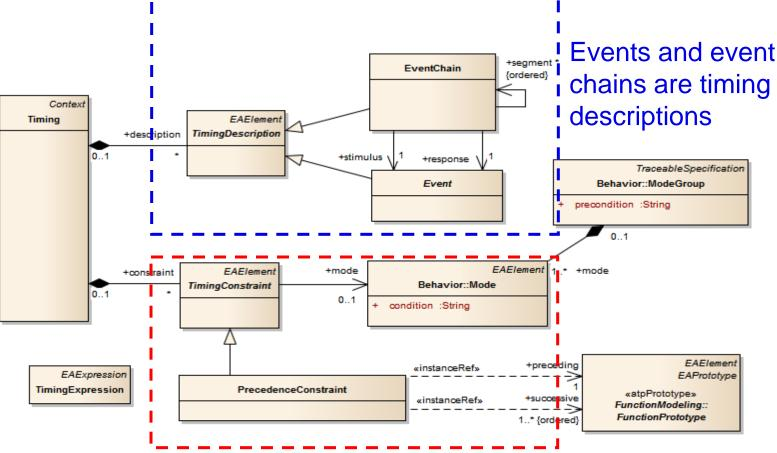
Timing constraints, imposed on events and event chains. The timing constraint is only valid when the specified mode is active EAST-ADL support for Timing
